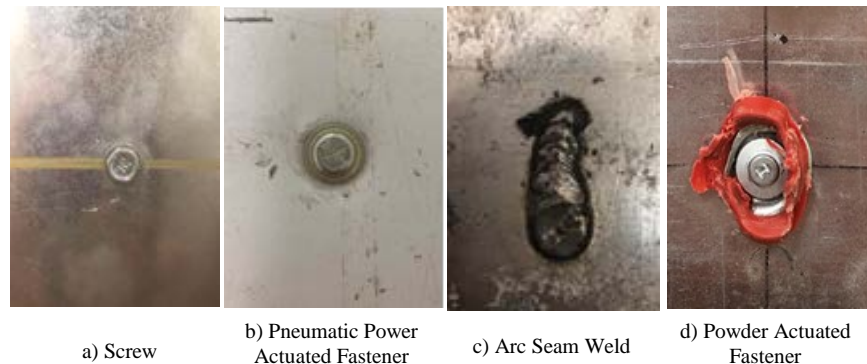
Figure 3. Picture of Each Type of Fastener Tested
